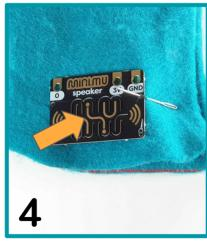
Sew the speaker to the glove with four little stitches through the holes around the edge.
