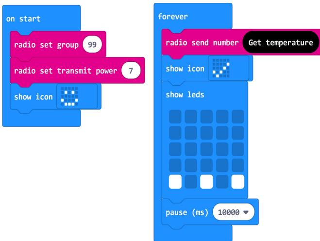
5. This is it for the first micro:bit. Once you've copied the code across, push on the enviro:bit, attach a battery pack, pop the whole thing in a food bag or a sandwich box, and find somewhere safe to put it outside. (We started with a sandwich box but it also worked with a Loot Box and we confused the birds!)
