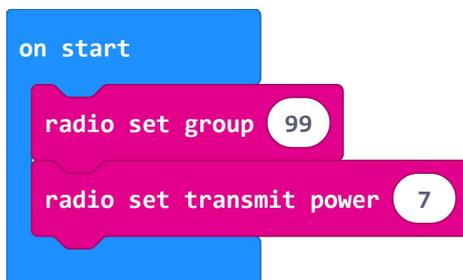
The transmit power goes up to 7, which is how strongly the signal is sent. If your micro:bits are right next to each other, you could turn this down to save power, but since ours is on the other side of the window, we've set it to full power.
